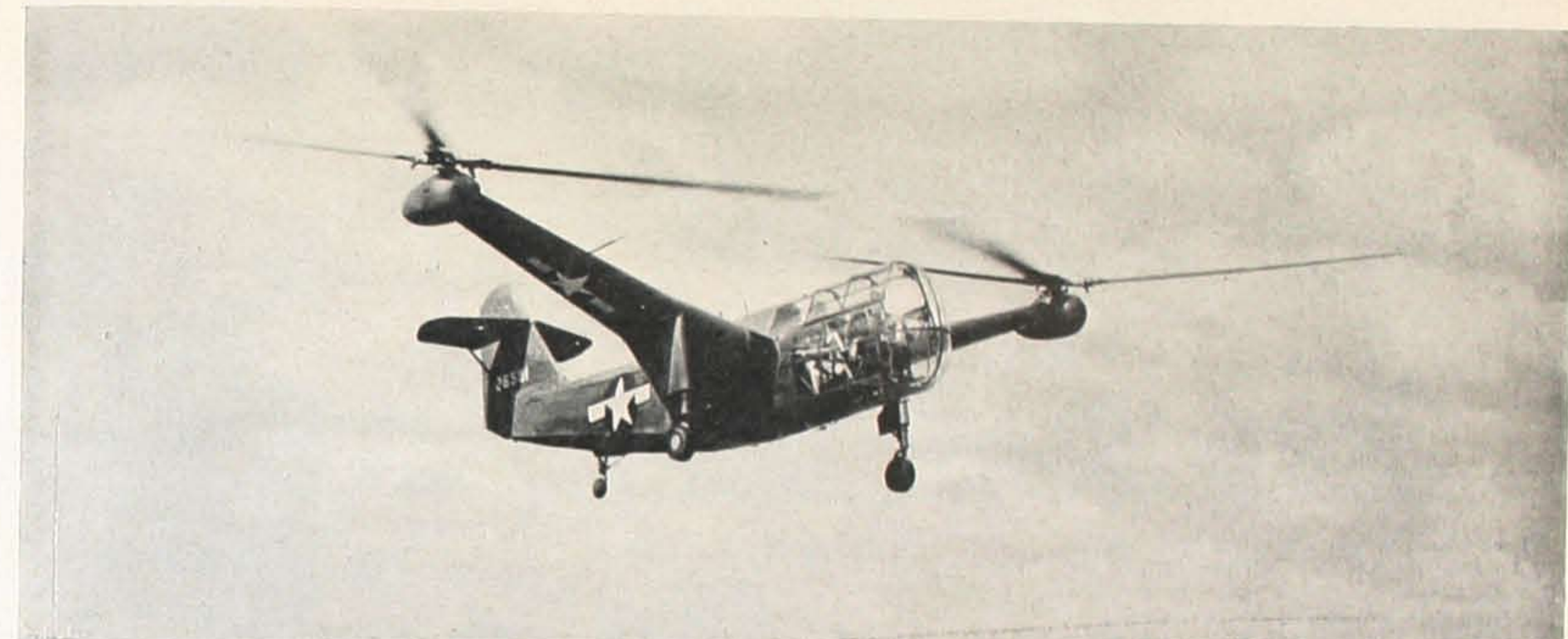
PLATT-LEPAGE HELICOPTER —"XR-1A" by Platt-LePage Aircraft Company. This is a military version powered with a 450 hp Pratt-Whitney engine. It has a tandem seating arrangement for pilot and observer. No production of commercial machines is contemplated at this time.
