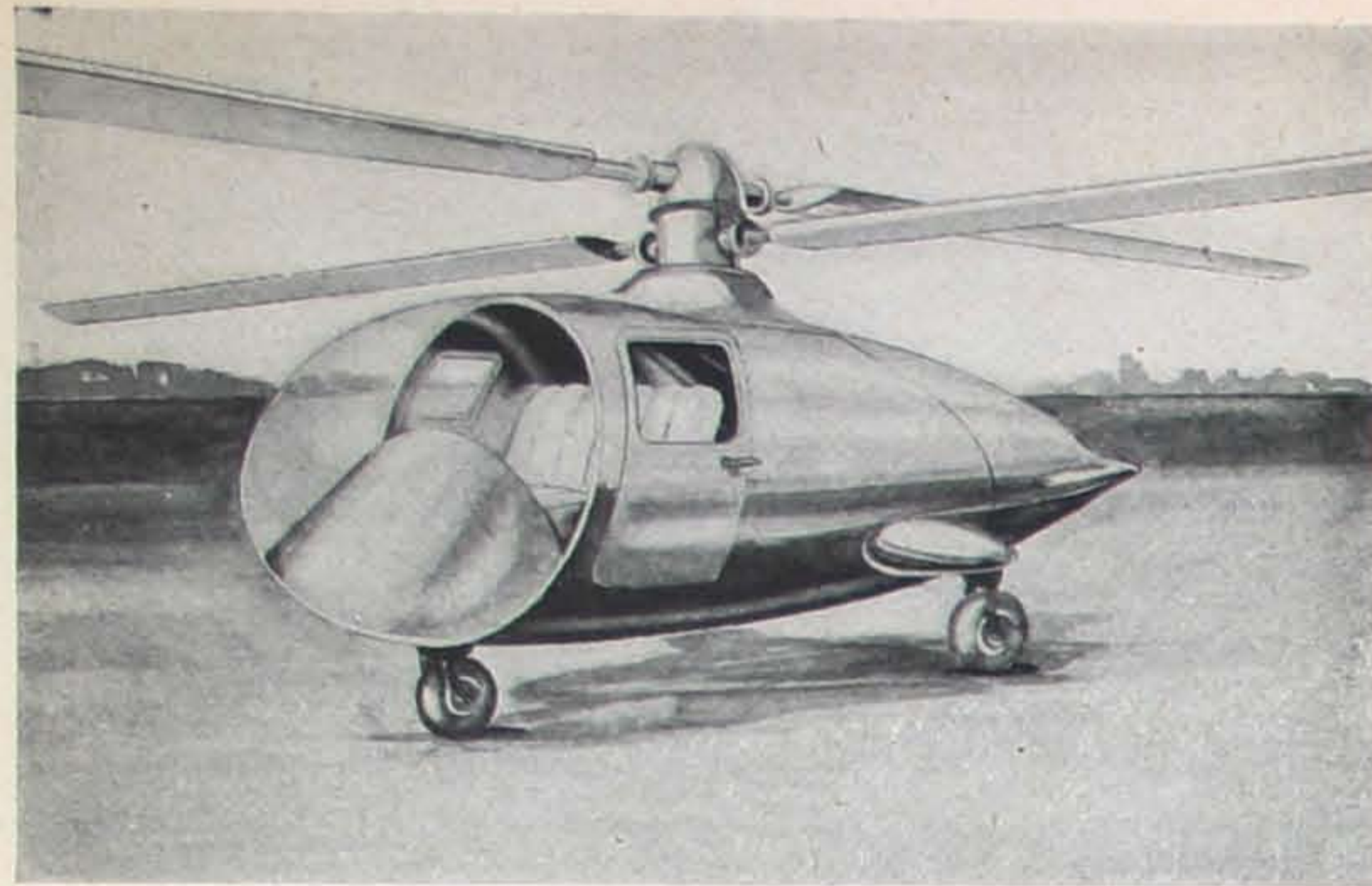
BURWELL HELICOPTER —Being developed in Toronto, the machine embodies a new type of control system whose main features are that the collective pitch lever, cyclic pitch stick, and rudder pedals operate a single control unit which is connected to the four rotor blades. No anti-torque rotor is needed, since the blades contra-rotate. A horizontally mounted opposed type engine of 150 hp drives 27 ft. rotor blades.
