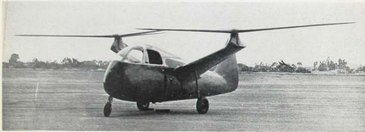
LANDGRAF HELICOPTER —A single-seater, powered by an 85 hp Pobjoy engine, speeds near 100 mph. Note retractable tricycle landing gear. Developments on additional models are in progress.
