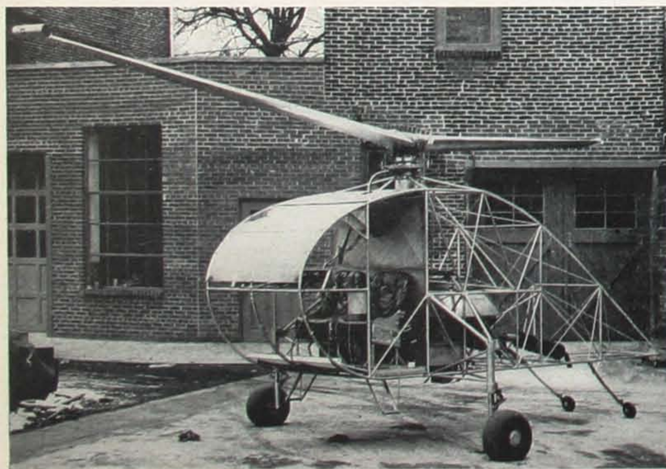
DE CHAPPEDELAINE HELICOPTER —Experimental model, a flow control rotor will be installed in which the boundary layer section of the airstream will be controlled to provide more efficient lift. Due to this and free floating rotor mounting, the control stick will lock in any position, enabling the craft to fly "hands off."
