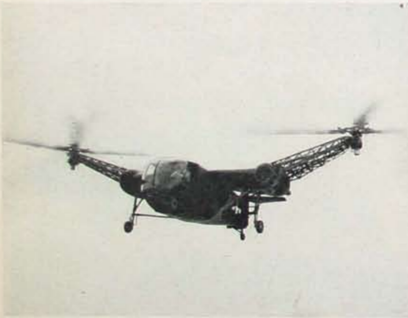
LANDGRAF HELICOPTER —A single-seater, powered by an 85 hp Pobjoy engine, speeds near 100 mph. Note retractable tricycle landing gear. Developments on additional models are in progress.
