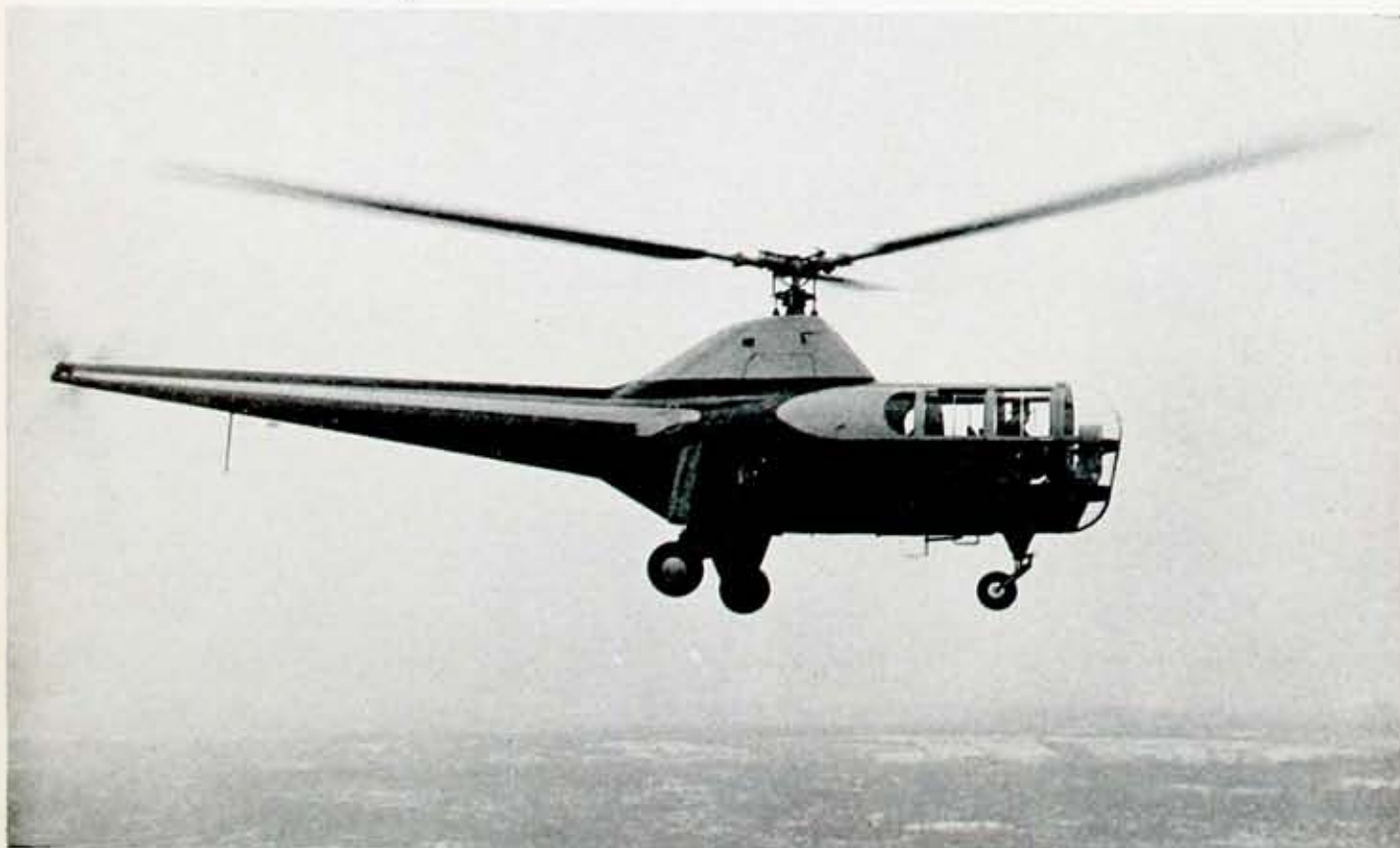
SIKORSKY AIRCRAFT—"S-51," Sikorsky helicopter shown here carries 3 passengers plus pilot. Powered by a Pratt-Whitney Wasp Junior R-985 engine, it has a maximum speed of slightly over 100 mph and will cruise at 80 mph. The S-51 succeeds the R-4B, R-5, and R-6 helicopters.
