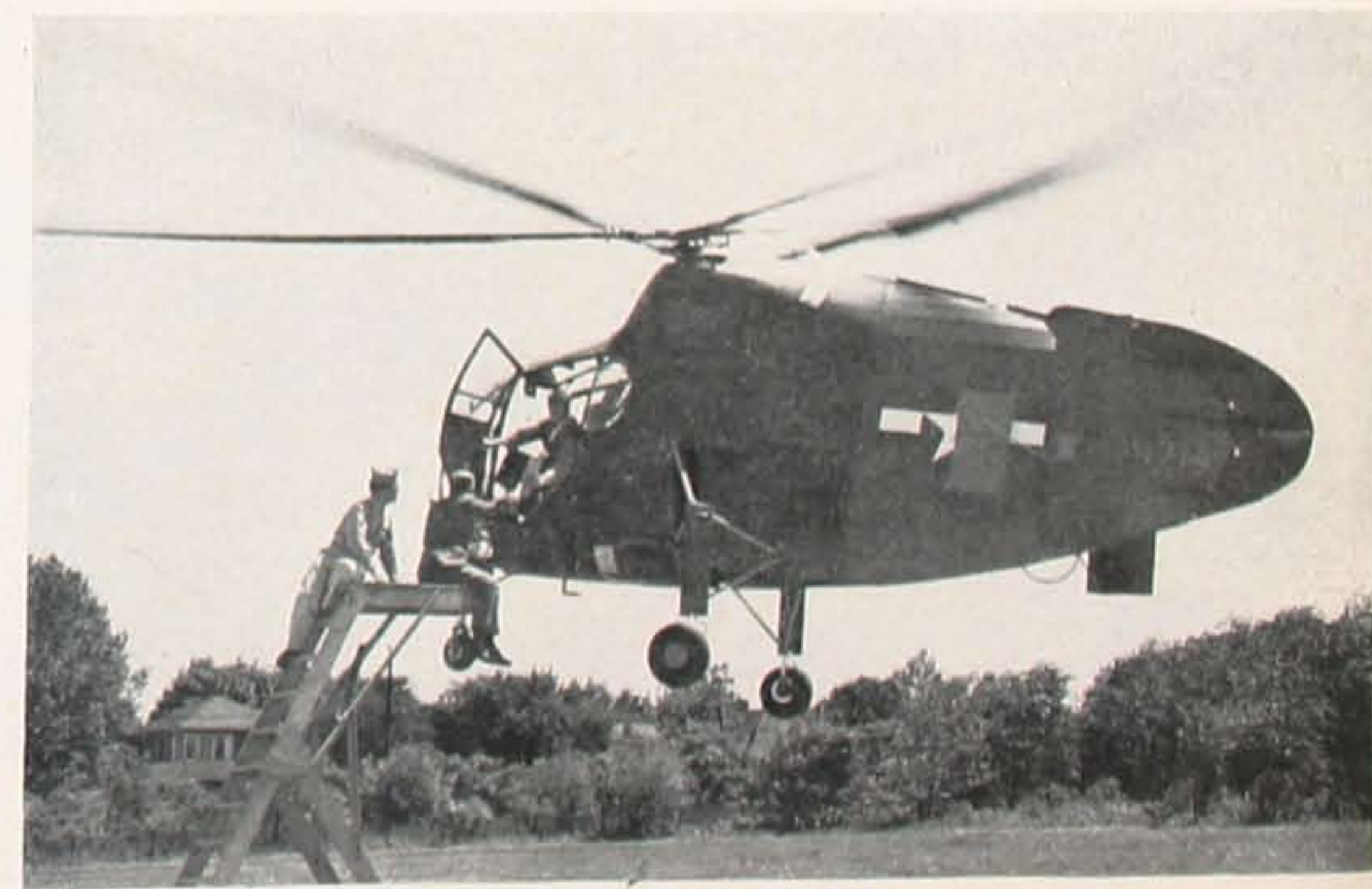
KELLETT AIRCRAFT —"XR-8" now undergoing flight tests, is powered by a 6 cylinder Franklin engine and incorporates the principle of intermeshing rotor blades.
