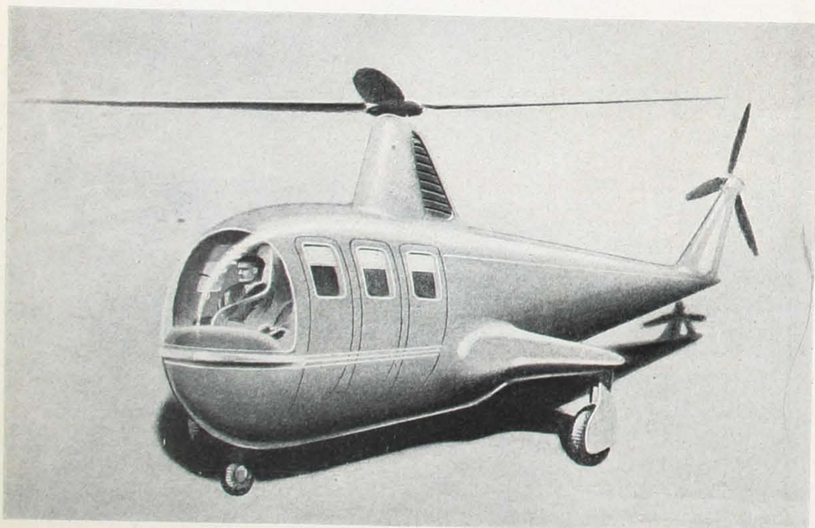
ROTAWINGS, Inc. —"Rota Airbus RA-2," will carry 7 passengers in addition to pilot. Speed is estimated at 115 to 120 mph with a cruising speed of 100 mph. Vertical climb rate is 450 fpm with a 10,000 ft. service ceiling. The "RA-2" will be powered by two Jacobs engines of 300 hp.
