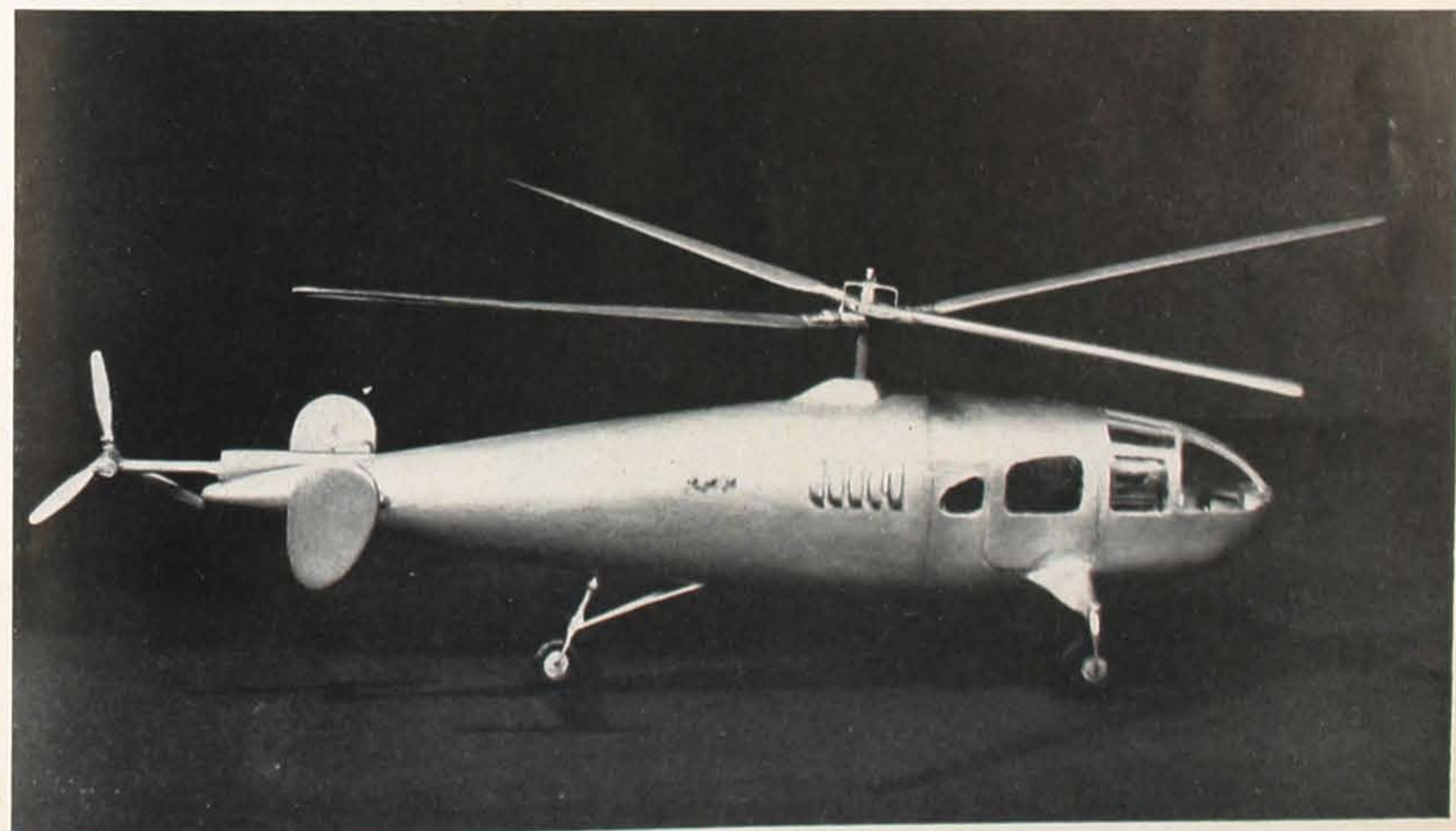
ENGINEERING PRODUCTS OF CANADA —The first Canadian helicopter, a three-place SG model VI, is powered by a Franklin, 6 cylinder, 178 hp motor at 3150 rpm. Gross weight 2218 lbs., weight empty 1550 lbs. It incorporates a four-bladed rotor with flapping and lag hinges and a four-bladed, semi-rigid see-sawing counter-torque rotor. Maximum speed 105 mph, cruising speed 80 mph, and cruising radius 160 miles.
