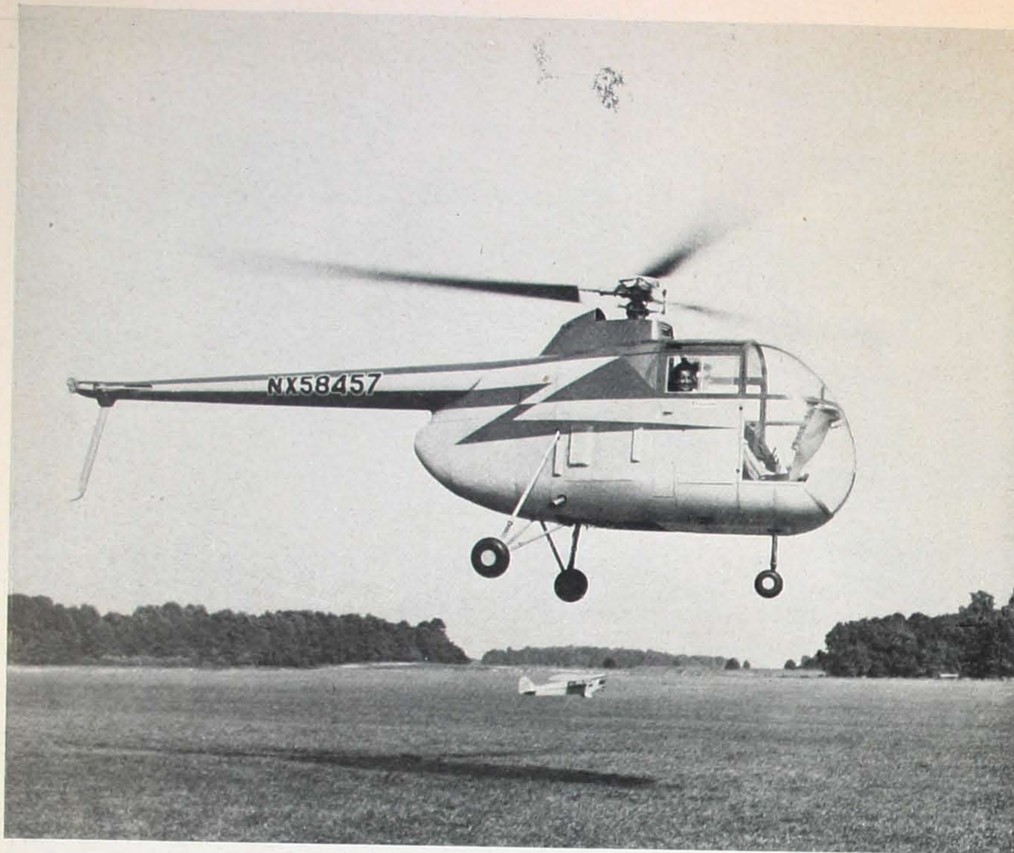
FIRESTONE HELICOPTER —The new two-place Model "45," powered by a small 125 hp four cylinder engine, incorporates a three-bladed main rotor and anti-torque tail rotor. Overall height is 8 ft. 1 in., length 25 ft. 5 in. It is equipped with dual controls, side-by-side seating arrangement in a lucite-enclosed cabin giving a 270 degree range of vision. Weighing less than a low-priced car, it can be flown hands-off controls.
