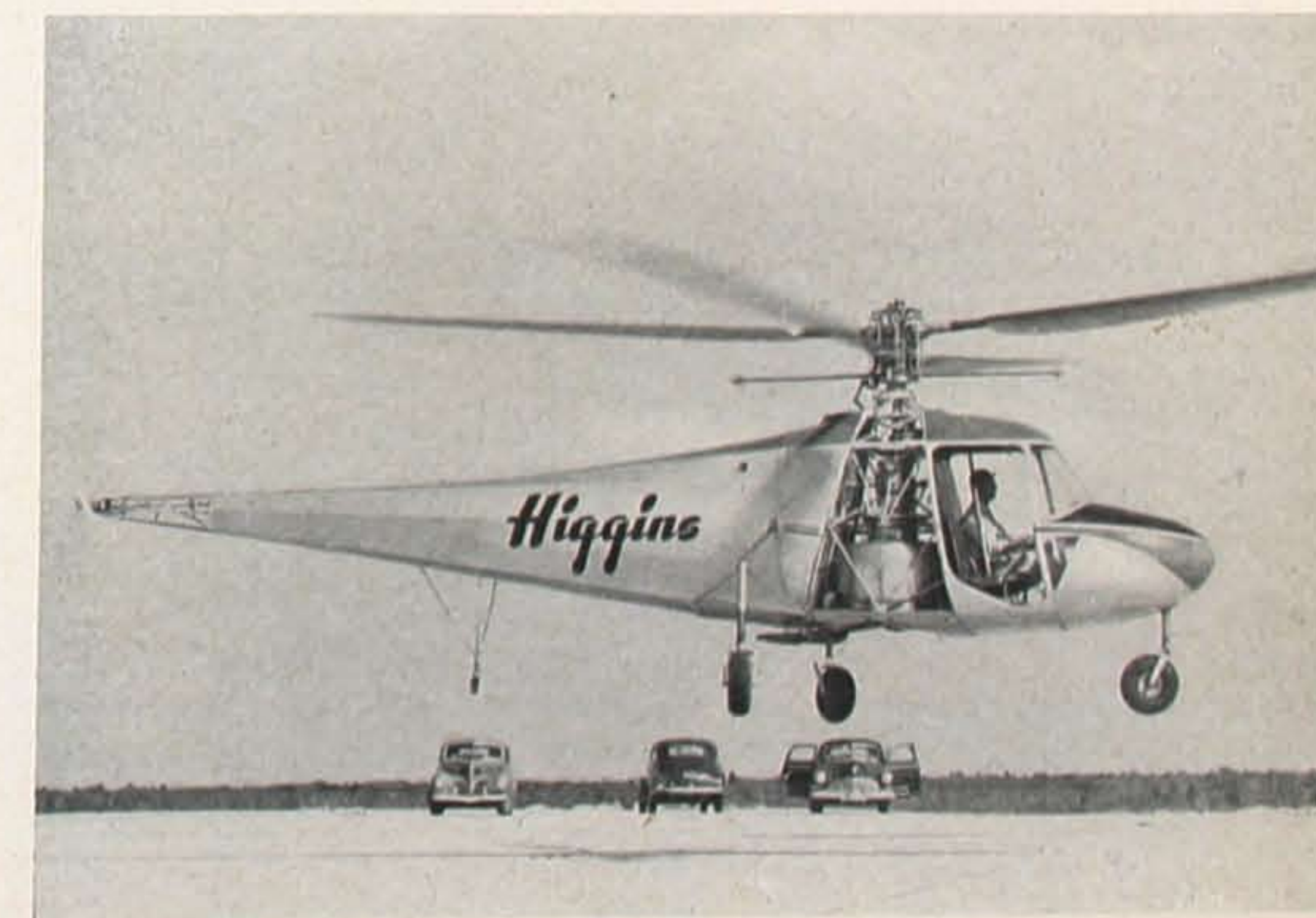
HIGGINS HELICOPTER —Designed by Enea Bossi in 1943, the EB-1 was flown quite successfully for a great many hours. Powered by a Warner 190 hp motor, the four bladed two seater weighed 2550 loaded, and 1950 empty. It was built by Higgins Industries, Inc., under Bossi license, to evaluate certain design theories, and was finally "retired" not long ago.
