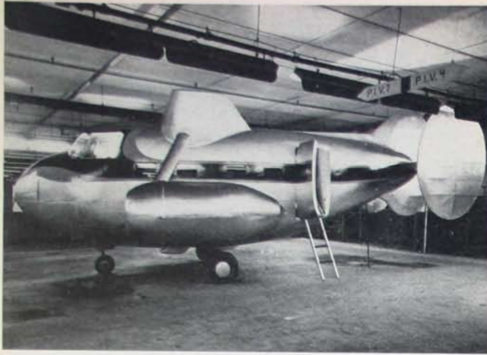
KELLETT AIRCRAFT — "KH-2," a large transport version of the proven inter-meshing configuration, with an engine in each compartment. The mock-up pictured here was under experiment for many months in an effort to develop an efficient cargo helicopter.
