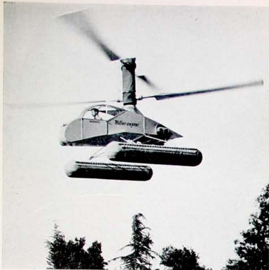
UNITED HELICOPTERS, Inc.—The new Hiller two-place Commuter model incorporates a two-bladed coaxial counter-rotating rotor system. It is powered by a 4 cylinder, 150 hp air-cooled engine. Rotors are provided with a chordwise flapping on see-saw hinge, classing it in the semi-rigid type. Blades can be lined up fore and aft for parking. The preliminary characteristics are as follows: gross weight 1600 lbs.; useful load 520 lbs.; maximum speed 100 mph., range 300 miles.
