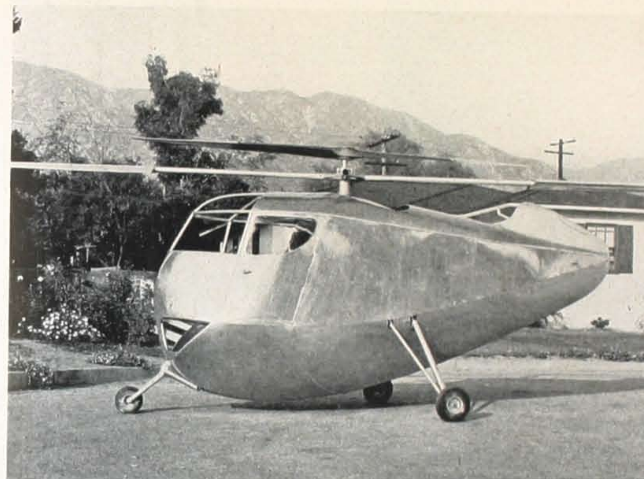
SAFTI-COPTER — This helicopter was designed to incorporate and simplify construction with many safety factors. Its size and shape are similar to the average automobile to utilize a minimum of storage space. Powered by a 40 hp Continental engine, the Safti-Copter will be economical to operate.
