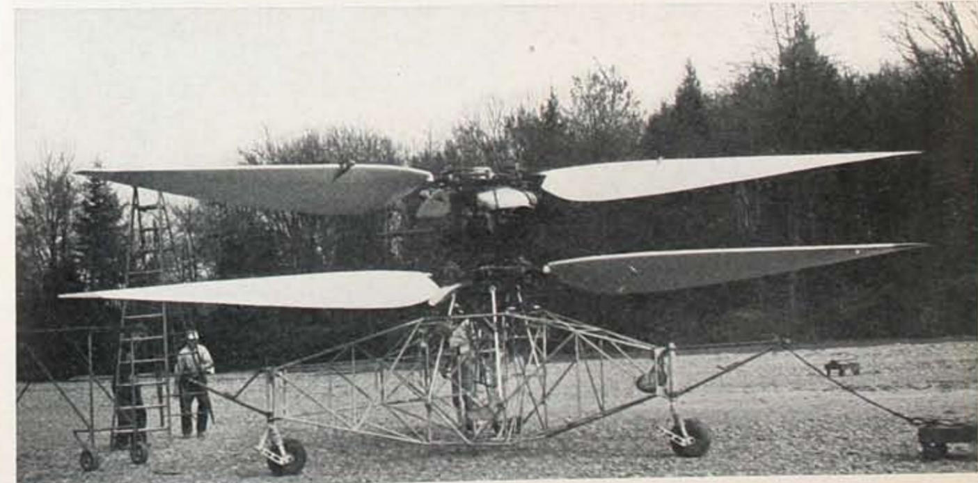
HELICOPTER CORPORATION OF AMERICA —The de Bothezat experimental model helicopter is of the coaxial type. It is equipped with a de Bothezat inter-airscrews helicopter engine of 75 hp, boosted to 80 hp. Airscrew diam. is 28'. Actual lift achieved in tests was over 20 lbs. per hp.
