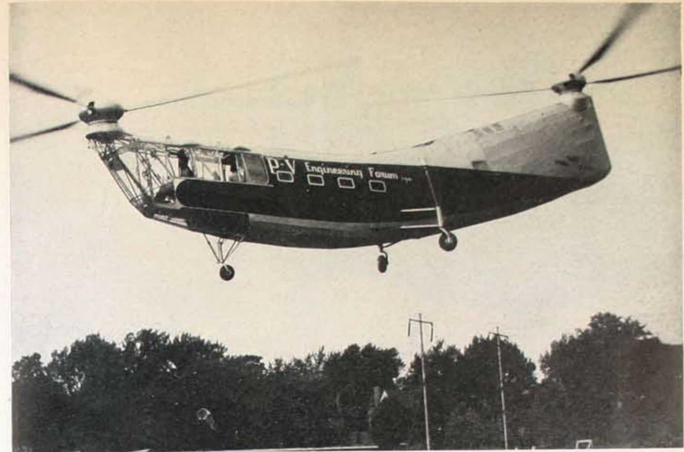
PIASECKI HELICOPTER —The "PV-3" manufactured by Piasecki Helicopter Corporation, is designed to carry 14 passengers in commercial operation. This is a development of the one-place "PV-2" still in operation after three years of intensive testing and demonstration.
