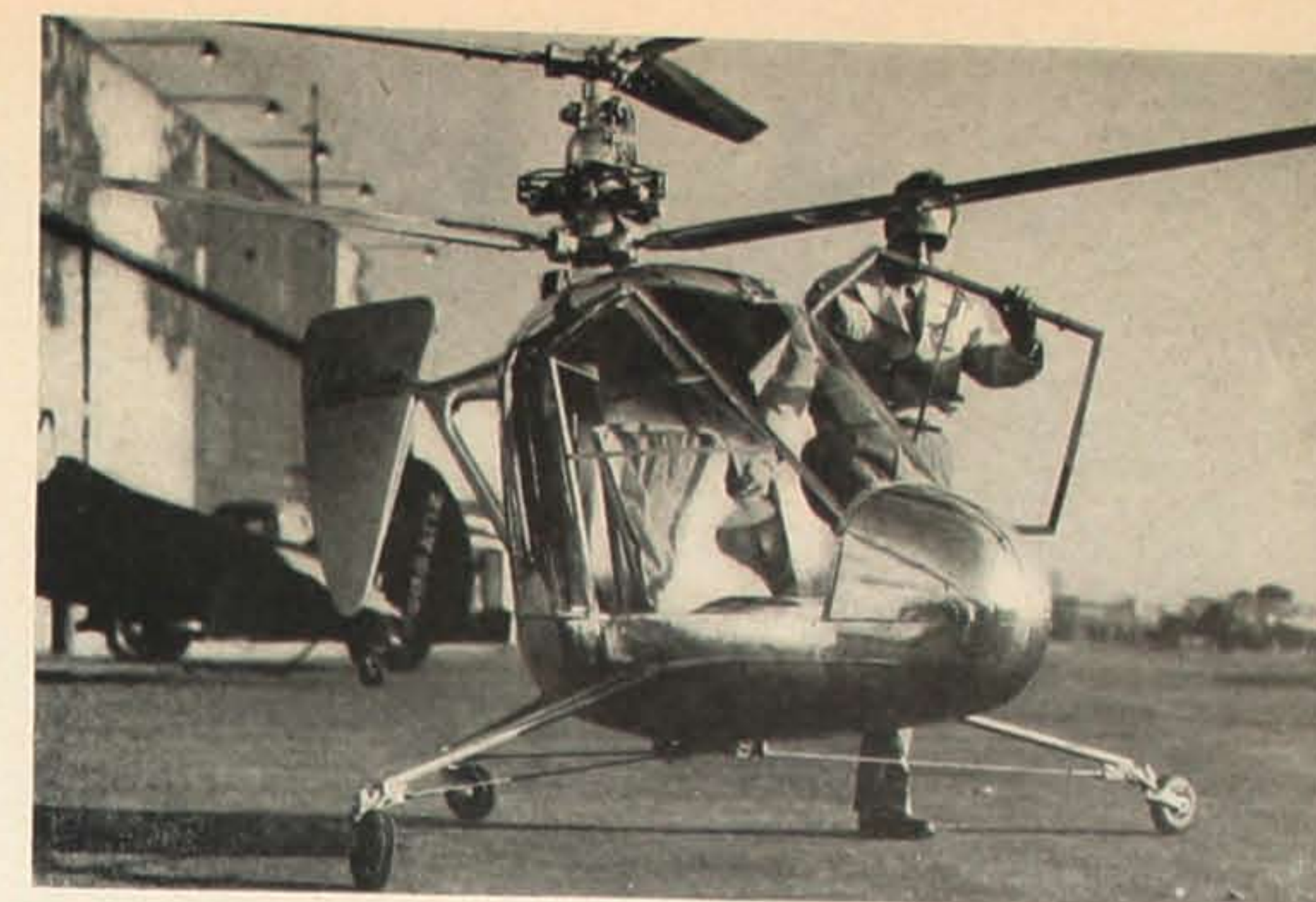
ROTERON —Roteron "X-100" is a small, safe, easily controlled and inexpensively operated helicopter. It incorporates coaxial rotors which go into autorotation if power fails. The price range will be about $2,800 in limited production, but will be less for mass production. Further specifications have not been released as yet.
