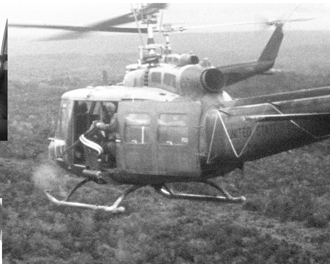
Door gunners started out using bungee straps to hold their M-60 machine guns. Later, they were given mounts.
